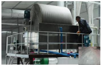
De-watering the pure starch milk to low water content of 35-40% by principle of vacuum suction filtration. Ensure sufficient water has been removed, otherwise the starch will form into lumps during drying.
