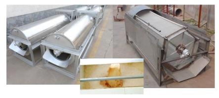
Commonly physical operation to separate fine cassava residues from cassava slurry. Oversize particles of cassava residues cannot pass through the lattice structure of the
