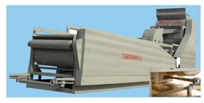
Crushing the peeled cassava roots into slurry and separate to remove the coarse cassava residues to obtain uniformly smooth cassava slurry. The crushing drum and all food contact areas should be made from stainless steel.
