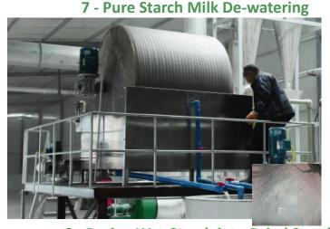
De-watering the pure starch milk to low water content of 35-40% by principle of vacuum suction filtration. Ensure sufficient water has been removed, otherwise the starch will form into lumps during drying.
