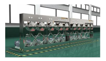
Solid control equipment that separate tiny sand and mud from the raw starch milk. De-sander is installed before the de-silter and normally the solids diameter for de-sander to be separated would be larger than for de-silter.
