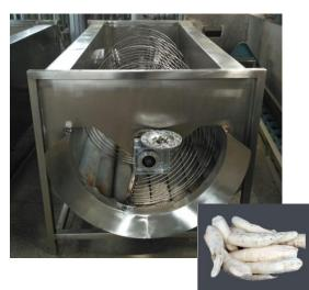
Peel the washed cassava roots to remove the outer brown skin and inner thick cream layer. The water source should be checked regularly to ensure it is not dirty or contaminated.
