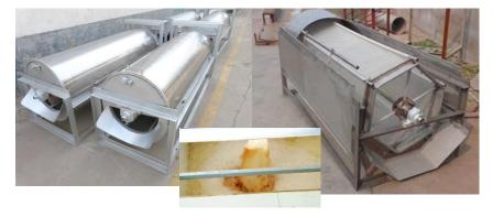
5 - Raw Starch Milk Desanding and Desilting:
