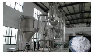
Effectively dry the wet starch into dried starch(tapioca) with low moisture content by principle of heat transfer exchange. The drying process is more reliable and of higher quality.
